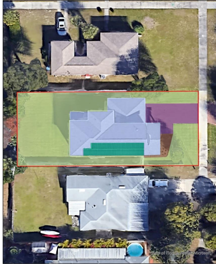
Figure 5-4. Parcel 17-31-16-23634-018-0080. This NS-2 parcel has the lowest solar reflectivity scores overall, with 0.20 for both vegetation and no vegetation scores. Solar panels are designed to absorb sunlight, not reflect it. The presence of solar panels on an already unreflective roof, and the presence of a painted driveway are likely responsible for the low score.
